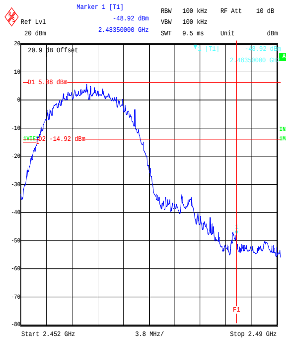
Title: EZURIO 2.4 GHz WLAN Module. FCC Part 15.247 Cond. BandEdge Comment A: 48271JD05 Top Channel DSSS QPSK Date: 8.SEP.2006 16:29:35
