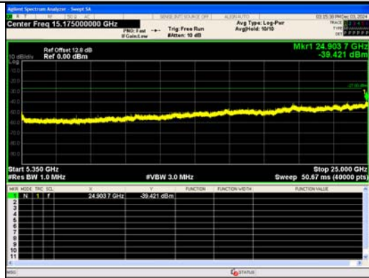
Spurious Emission:5350~25000.0 MHz IEEE 802.11ac Channel 58 80MHz Antenna 0
