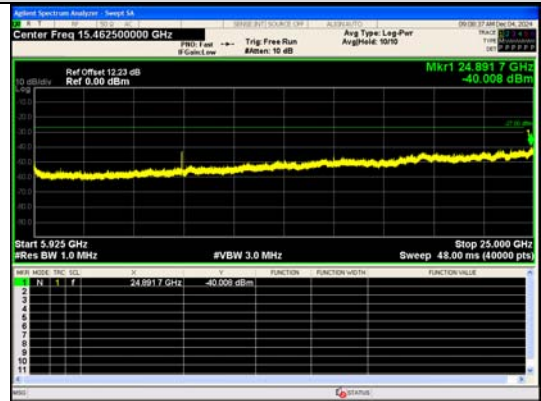
Spurious Emission:5925~25000.0 MHz IEEE 802.11ac Channel 157 20MHz Antenna 0
