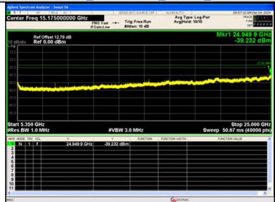
Spurious Emission:5350~25000.0 MHz IEEE 802.11n Channel 36 20MHz Antenna 0
