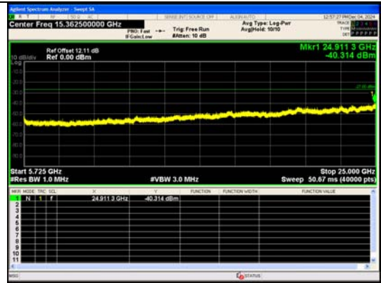
Spurious Emission:5725~25000.0 MHz IEEE 802.11n Channel 100 20MHz Antenna 0
