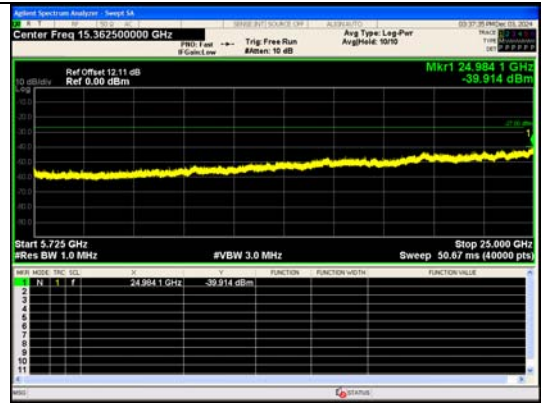
Spurious Emission:5725~25000.0 MHz IEEE 802.11ac Channel 100 20MHz Antenna 0
