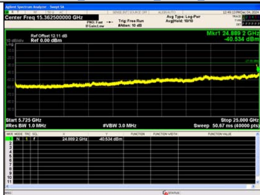
Spurious Emission:5725~25000.0 MHz IEEE 802.11a Channel 100 20MHz Antenna 0
