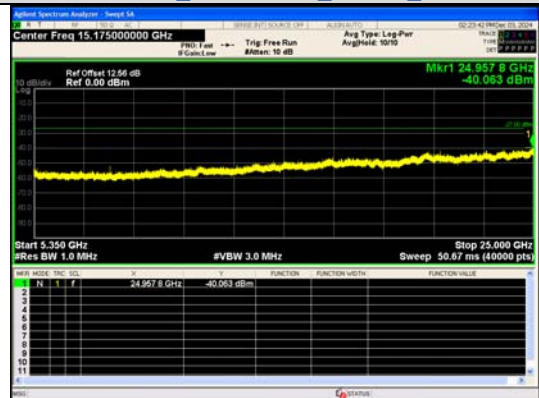
Spurious Emission:5350~25000.0 MHz IEEE 802.11ac_Channel 42_80MHz_Antenna 0
