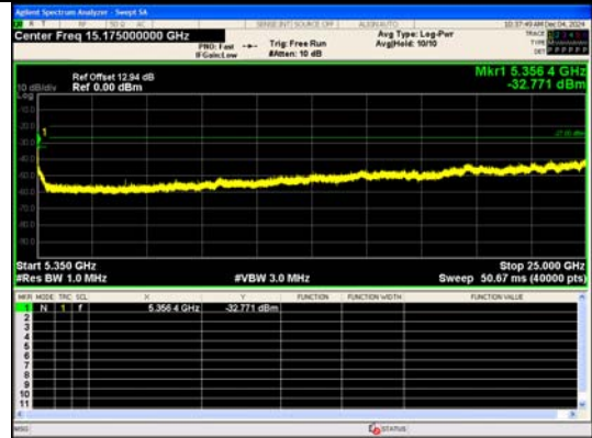
Spurious Emission:5350~25000.0 MHz IEEE 802.11a Channel 64 20MHz Antenna 0
