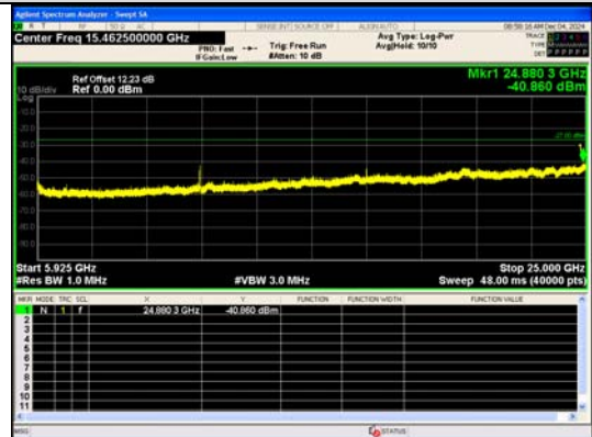
Spurious Emission:5925~25000.0 MHz IEEE 802.11a Channel 157 20MHz Antenna 0
