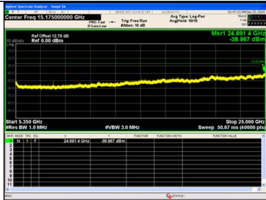
Spurious Emission:5350~25000.0 MHz IEEE 802.11ac Channel 40 20MHz Antenna 0
