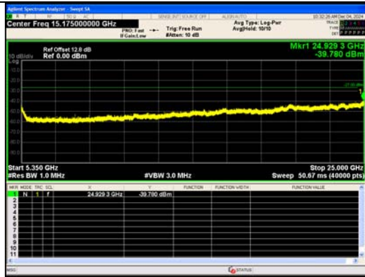
Spurious Emission:5350~25000.0 MHz IEEE 802.11a Channel 56 20MHz Antenna 0
