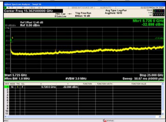
Spurious Emission:5725~25000.0 MHz IEEE 802.11n Channel 140 20MHz Antenna 0
