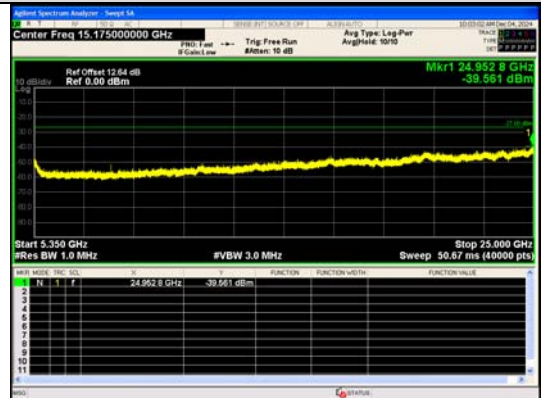
Spurious Emission:5350~25000.0 MHz IEEE 802.11n Channel 48 20MHz Antenna 0
