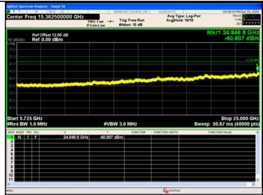
Spurious Emission:5725~25000.0 MHz IEEE 802.11ac Channel 106 80MHz Antenna 0
