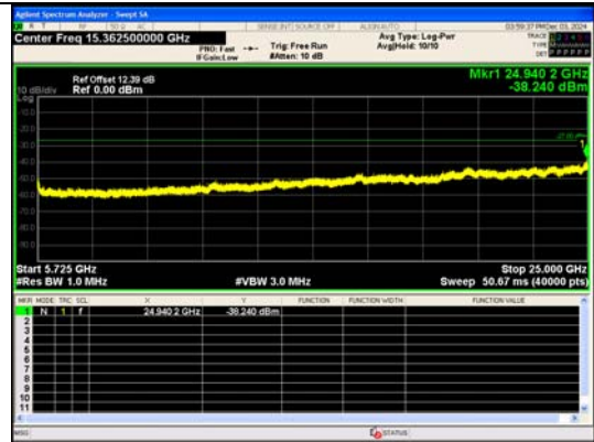
Spurious Emission:5725~25000.0 MHz IEEE 802.11ac_Channel 118_40MHz_Antenna 0
