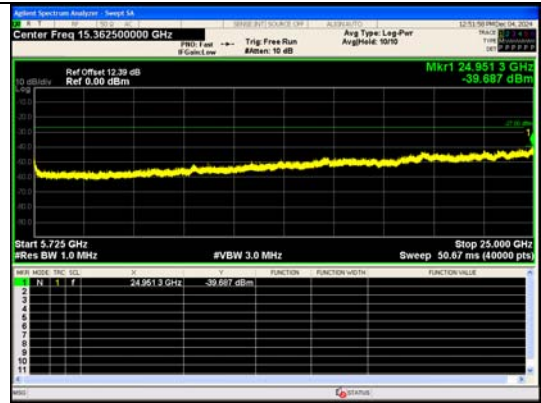
Spurious Emission:5725~25000.0 MHz IEEE 802.11a Channel 120 20MHz Antenna 0
