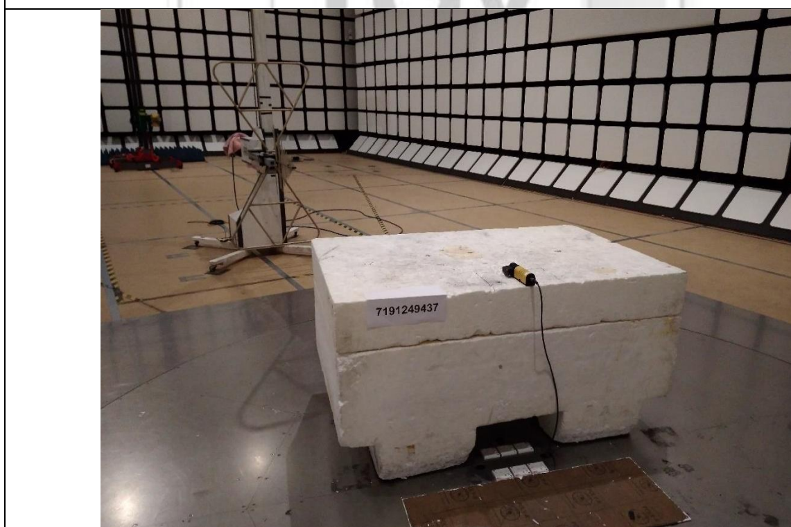
Radiated Emissions (Spurious Emissions Inclusive Restricted Bands Requirement) Test Setup (Rear View)
