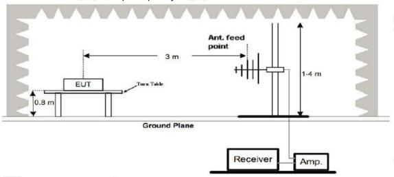
3. Radiated Emission Test-Up Frequency Above 1GHz
