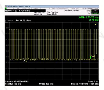
The graph shows the duration of 'on' signal. From marker 1 to marker 2, duration is 846 \mus.
