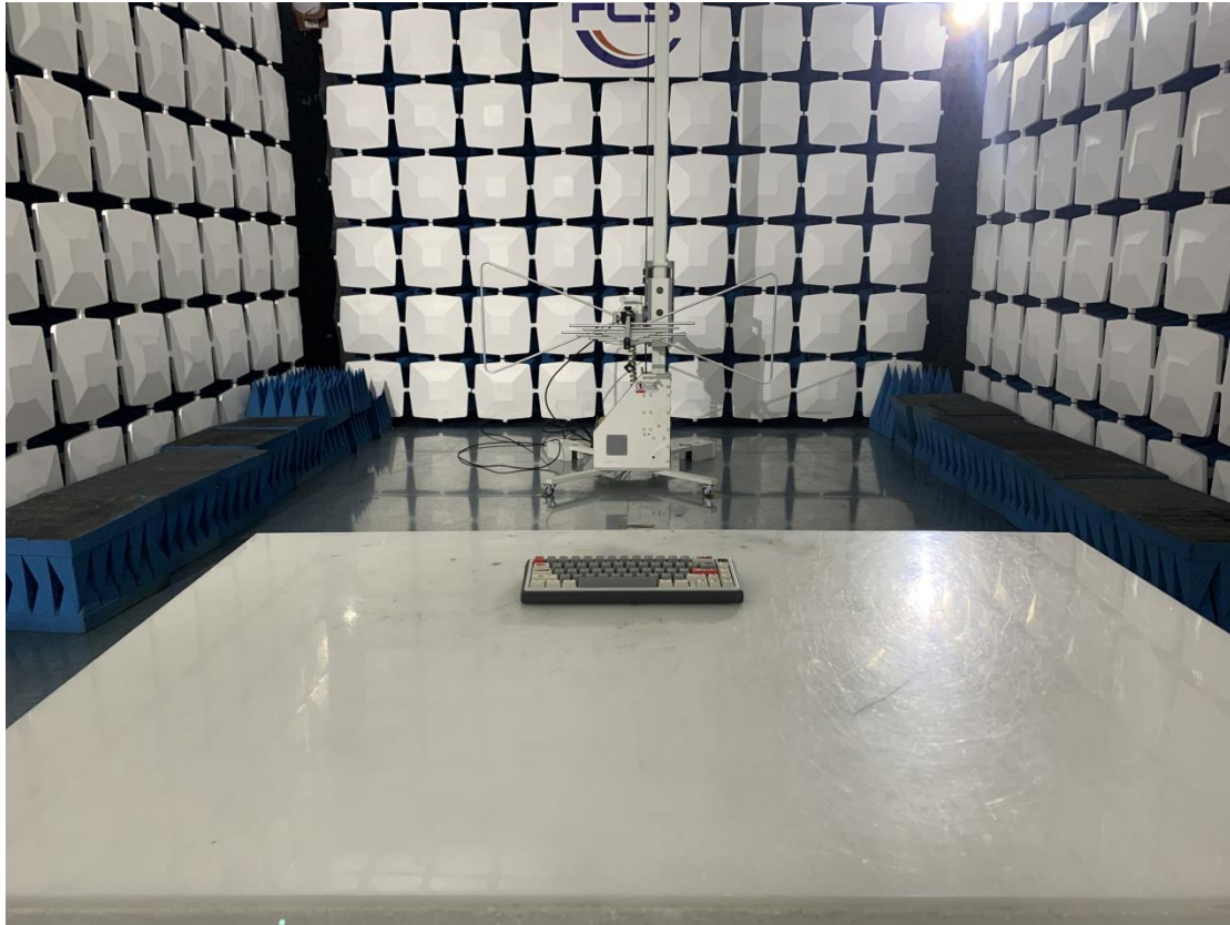
Blow 1GHz for radiated emission test setup
