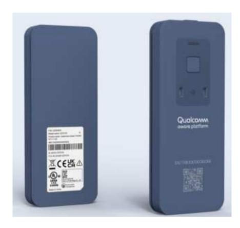
QTS110GW is a track and sense device that can be used in shipping and logistics field for tracking the location of a cargo and to monitor environmental condition of cargo during transit and during warehousing. The device can be used in multimodal journeys over land, sea and air.
