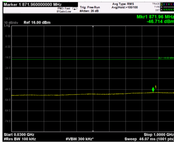
Channel: BOTTOM, Modulation: 64QAM, BW=15MHz, Range: Lower
