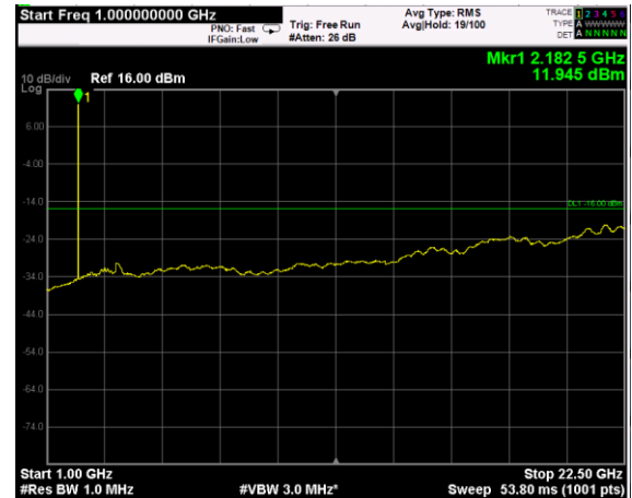
Channel: BOTTOM, Modulation: QPSK, BW=5MHz, Range: Upper
