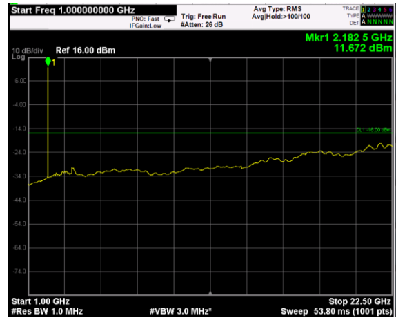
Channel: BOTTOM, Modulation: 256QAM, BW=5MHz, Range: Upper
