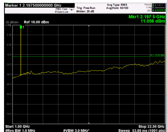
Channel: TOP, Modulation: QPSK, BW=5MHz, Range: Upper
