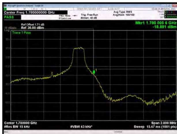
LTE Band 66 16QAM 1.4MHz CH-High, 100%RB
