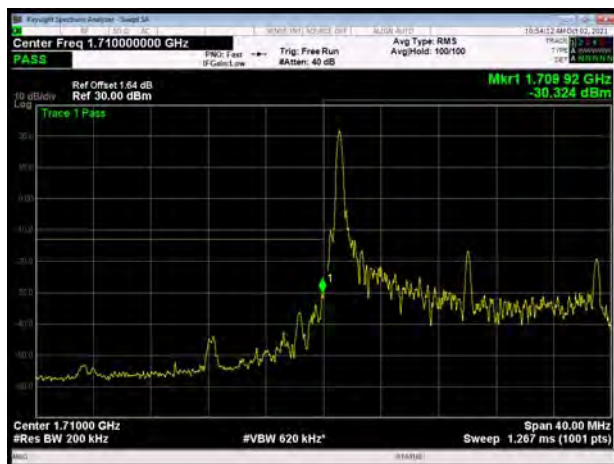
LTE Band 66 QPSK 20MHz CH-Low, 100%RB
