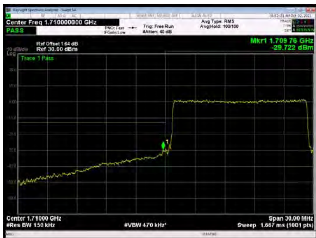
LTE Band 66 16QAM 20MHz CH-Low, 1 RB
