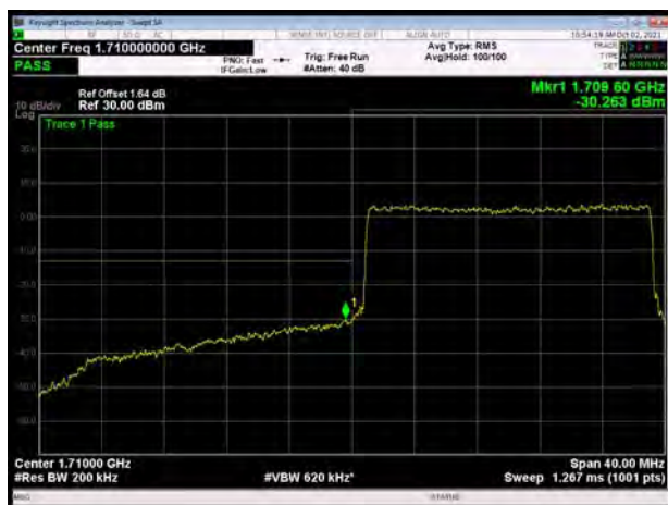
LTE Band 66 QPSK 20MHz CH-Low, 100%RB
