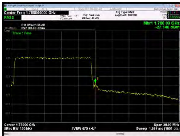
LTE Band 66 16QAM 20MHz CH-High, 1 RB
