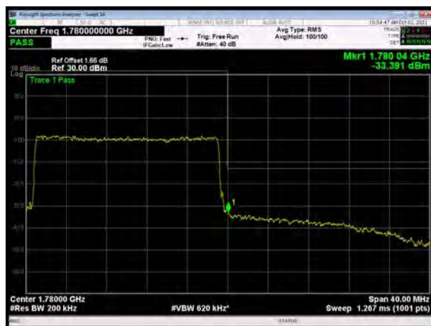
LTE Band 66 16QAM 20MHz CH-High, 100%RB
