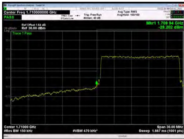
LTE Band 66 QPSK 20MHz CH-Low, 1 RB
