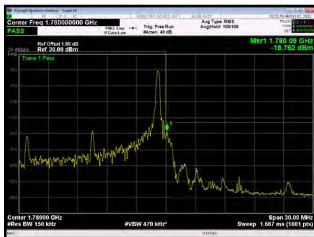
LTE Band 66 16QAM 15MHz CH-High, 1 RB
