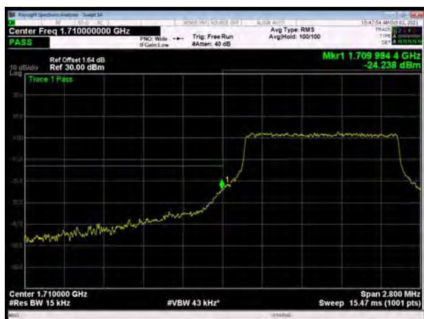
LTE Band 66 16QAM 3MHz CH-Low, 1 RB
