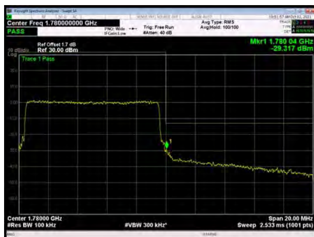
LTE Band 66 16QAM 15MHz CH-High, 1 RB
