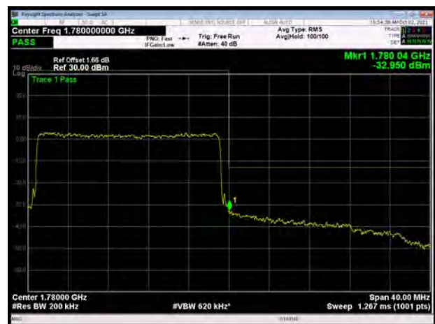
LTE Band 66 QPSK 20MHz CH-High, 100%RB
