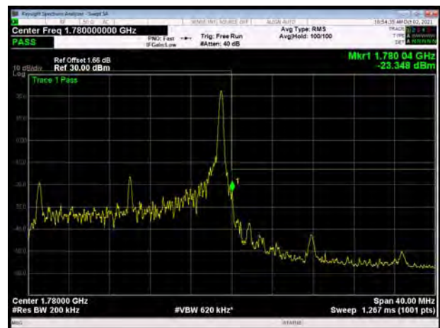
LTE Band 66 QPSK 20MHz CH-High, 100%RB
