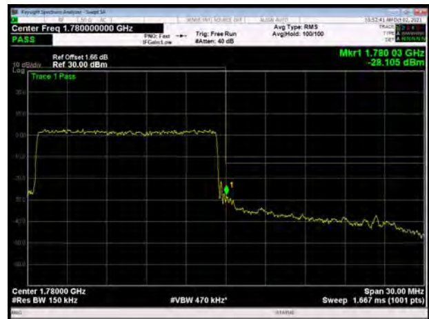
LTE Band 66 QPSK 20MHz CH-High, 1 RB
