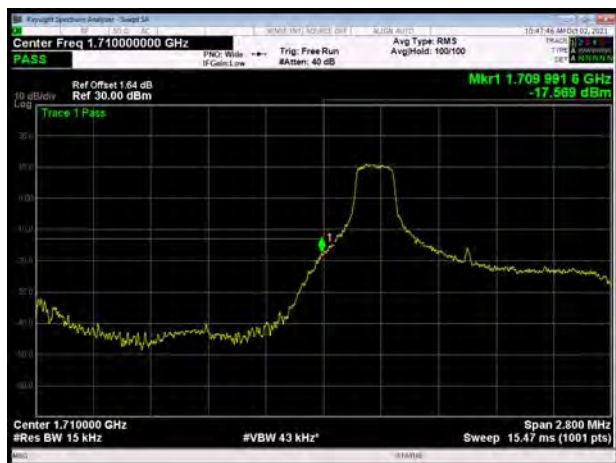
LTE Band 66 16QAM 1.4MHz CH-Low, 100%RB
