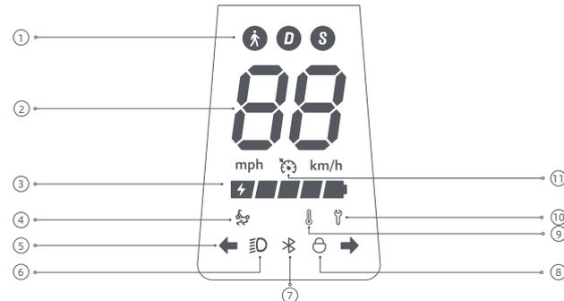
① Riding Modes:
