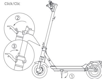
EN Put down the kickstand, and hold up the stem until it is completely in an upright position. Then push the quick release lever inward to the end.
