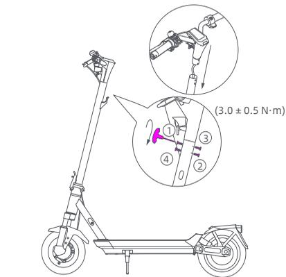
EN Install the handlebar onto the stem, and make sure to install the handlebar in the correct direction. Follow the number order as illustrated to pre-tighten the four screws with the included Allen key. Make sure the handlebar is correctly installed and then tighten the screws thoroughly.
