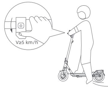
EN Step on the deck with one foot, and slowly kicks off the other on the ground. When the scooter starts to coast, put both feet on the deck and gently press the accelerator.
