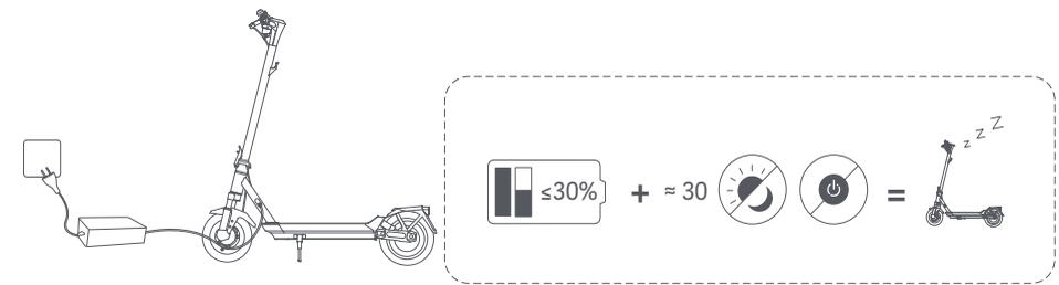
EN The scooter is fully charged when the LED on the battery charger changes from red to green.
