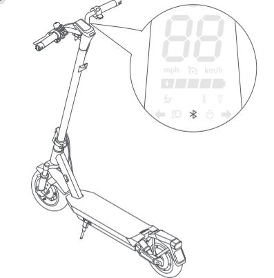
EN Power on the scooter; a blinking Bluetooth icon indicates the scooter is waiting to be connected.
