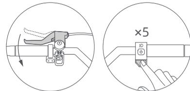
EN Turn the scooter on. Make sure the scooter is not locked or during charging, squeeze the brake lever and simultaneously press the accelerator 5 times, when the display is off, the scooter has been restored to factory settings, and the scooter cannot be searched for by the Find My app. If you need to pair again, delete the added scooter from the Find My app and then pair it again.
