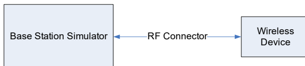
Figure 9-1 Power Measurement Setup
