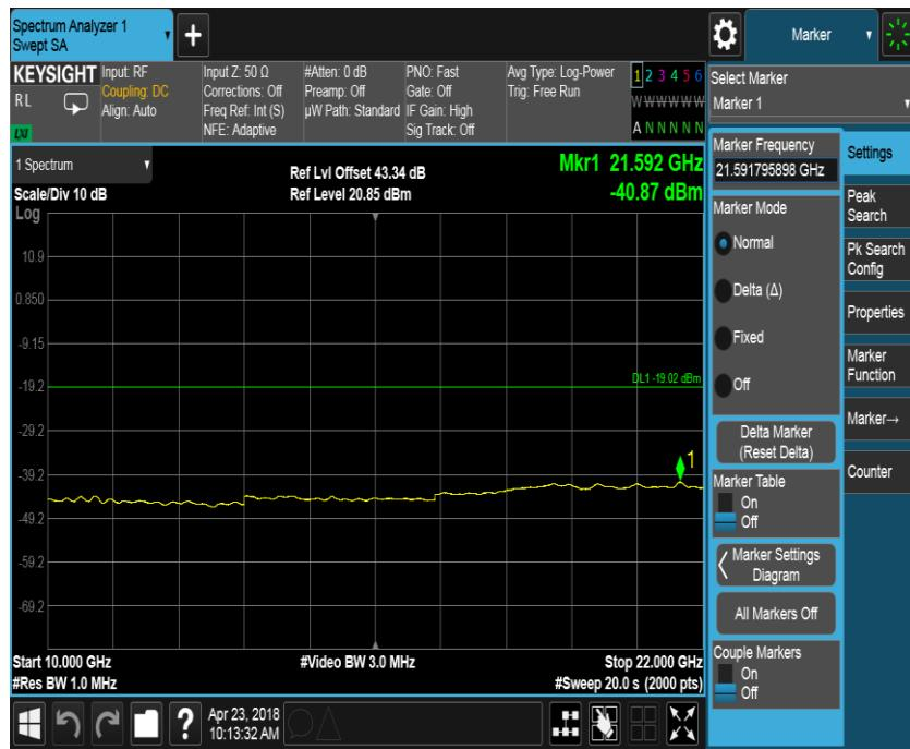
Port D, Channel Position M, LTE 5.0 MHz
