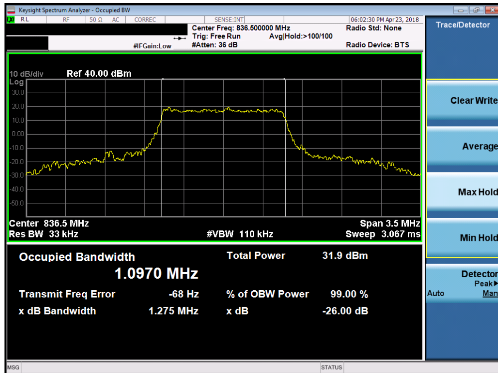
Plot 7-14. Occupied Bandwidth Plot (Band 5 – 1.4MHz 16-QAM - Full RB Configuration)
