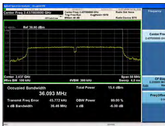
(802.11n40) 6dB Bandwidth plot on channel 9
