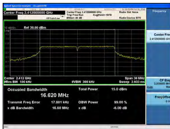
(802.11g) 6dB Bandwidth plot on channel 6
