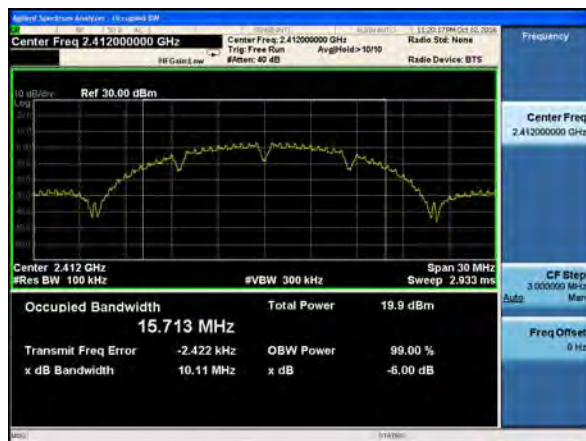
(802.11b) 6dB Bandwidth plot on channel 6
