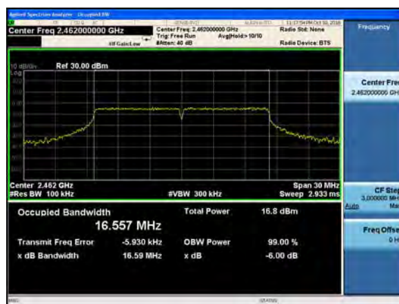
(802.11g) 6dB Bandwidth plot on channel 11
