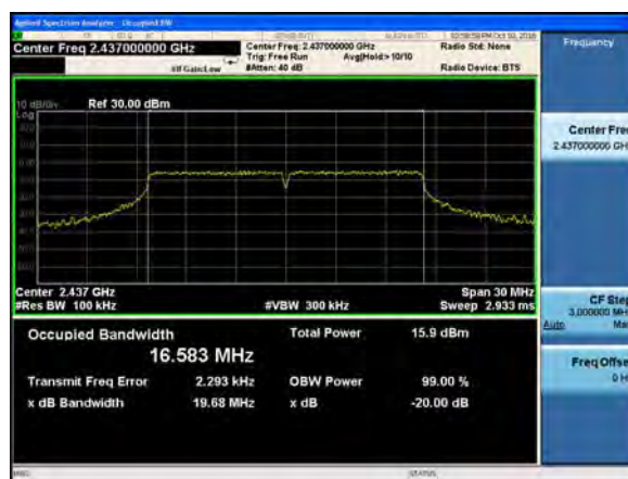
(802.11g) -20dB Bandwidth plot on channel 11
