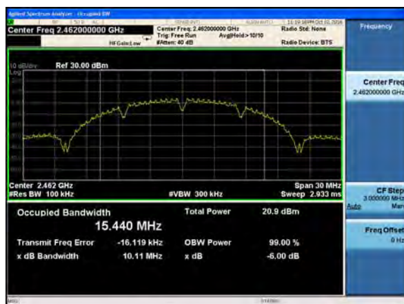
(802.11b) 6dB Bandwidth plot on channel 11
