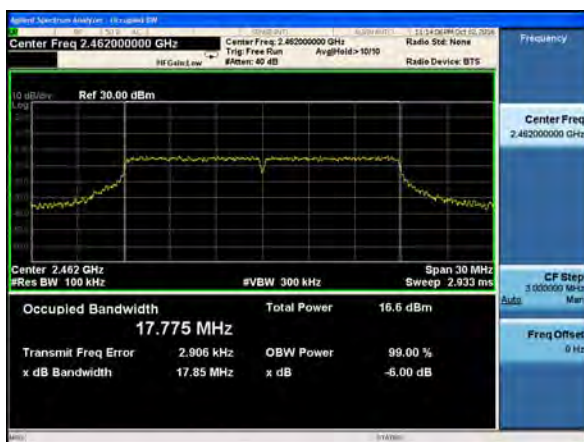
(802.11n20) 6dB Bandwidth plot on channel 11
