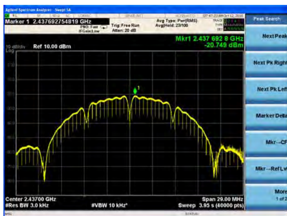
(802.11b) PSD plot on channel 11
