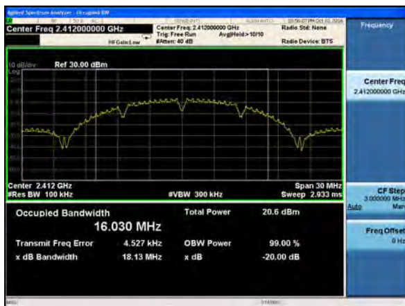
(802.11b) -20dB Bandwidth plot on channel 6
