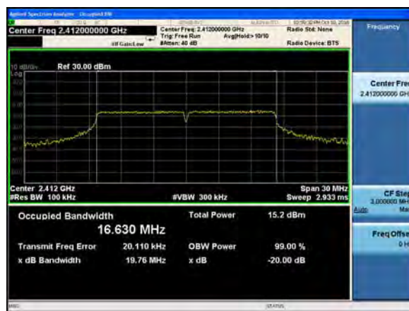
(802.11g) -20dB Bandwidth plot on channel 6
