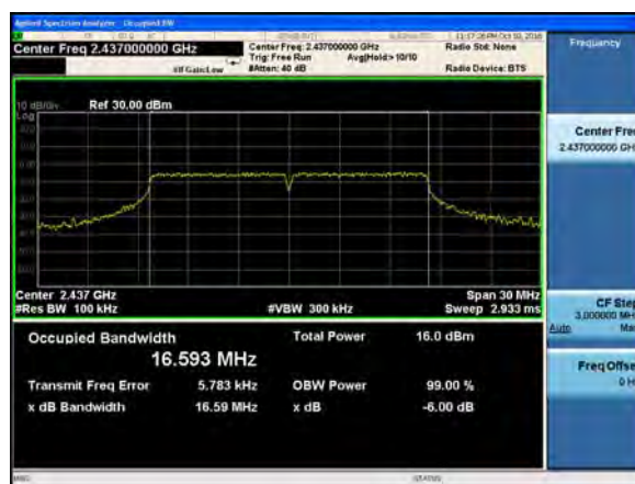
(802.11g) 6dB Bandwidth plot on channel 11
