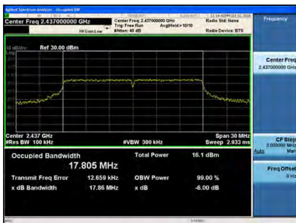
(802.11n20) 6dB Bandwidth plot on channel 11
