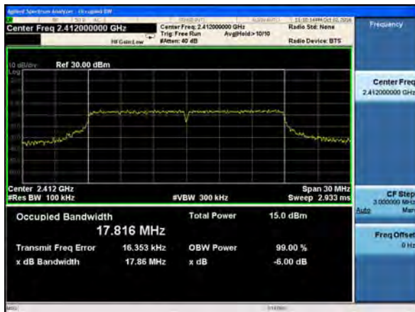
(802.11n20) 6dB Bandwidth plot on channel 6
