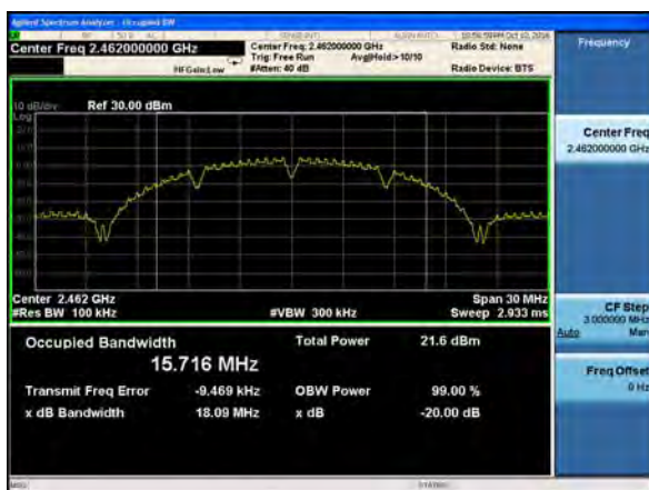
(802.11b) -20dB Bandwidth plot on channel 11
