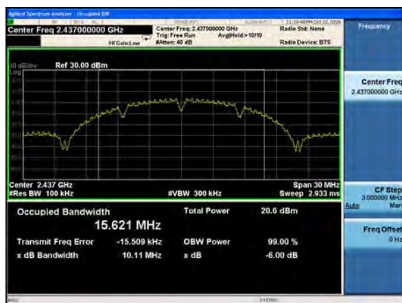
(802.11b) 6dB Bandwidth plot on channel 11
