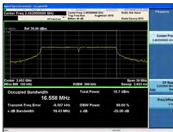
(802.11g) -20dB Bandwidth plot on channel 11
