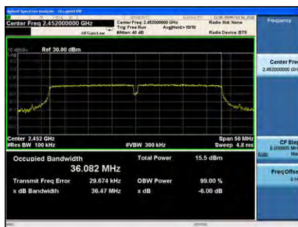
(802.11n40) 6dB Bandwidth plot on channel 9
