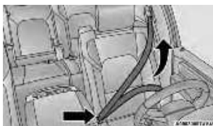
Positioning The Lap Belt
