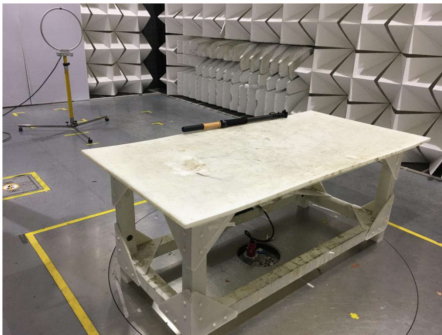
Radiated spurious emission Test Setup-1(Below 30MHz)
