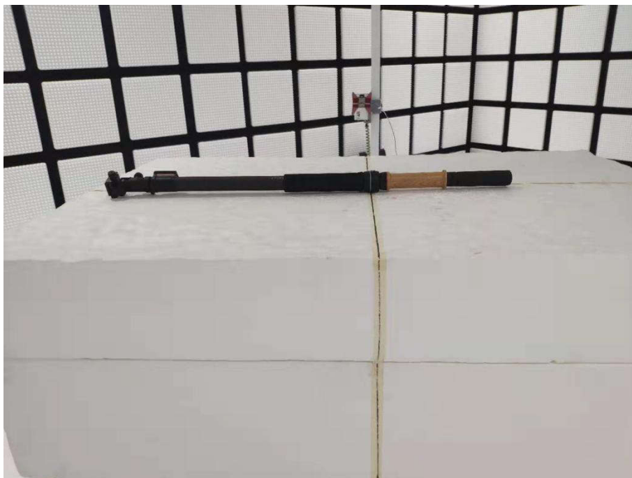
Radiated spurious emission Test Setup-3(Above 1GHz)
