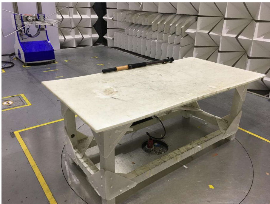
Radiated spurious emission Test Setup-2(Below 1GHz)
