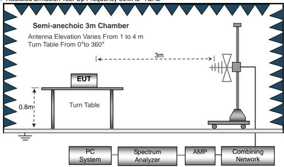
(C) Radiated Emission Test-Up Frequency Above 1GHz
