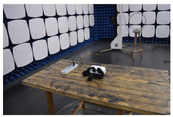
3. Radiated emission (9KHz-30MHz)
