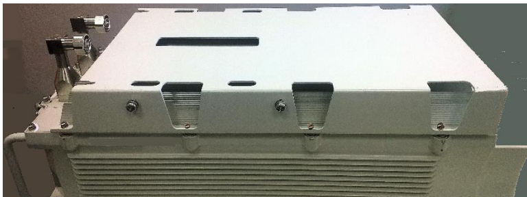
Figure 13: AirHarmony-4400 in Prone Position Prior to Front External Filter Assembly
