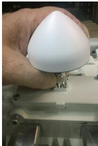
Figure 24: Attaching GPS antenna to unit
