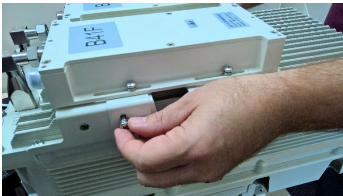
Figure 8: Mounting Rear External Filters' set
