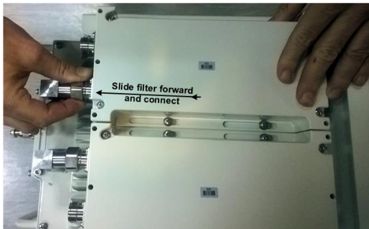
Figure 21: Align and fit second filter to connector
