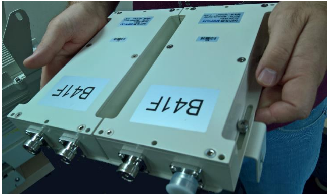
Figure 7: Rear External Filters' Set
