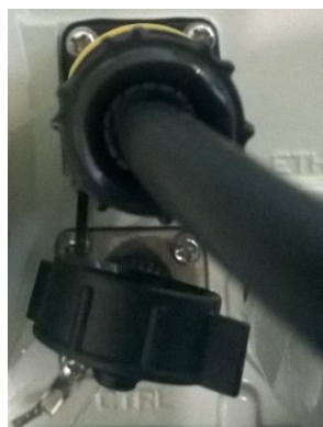
Figure 53: Power cable attached to AirHarmony-4400
