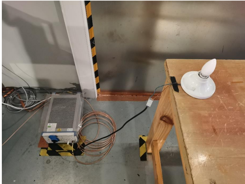
Photograph 2: Set-up for measurement of radiated emission
