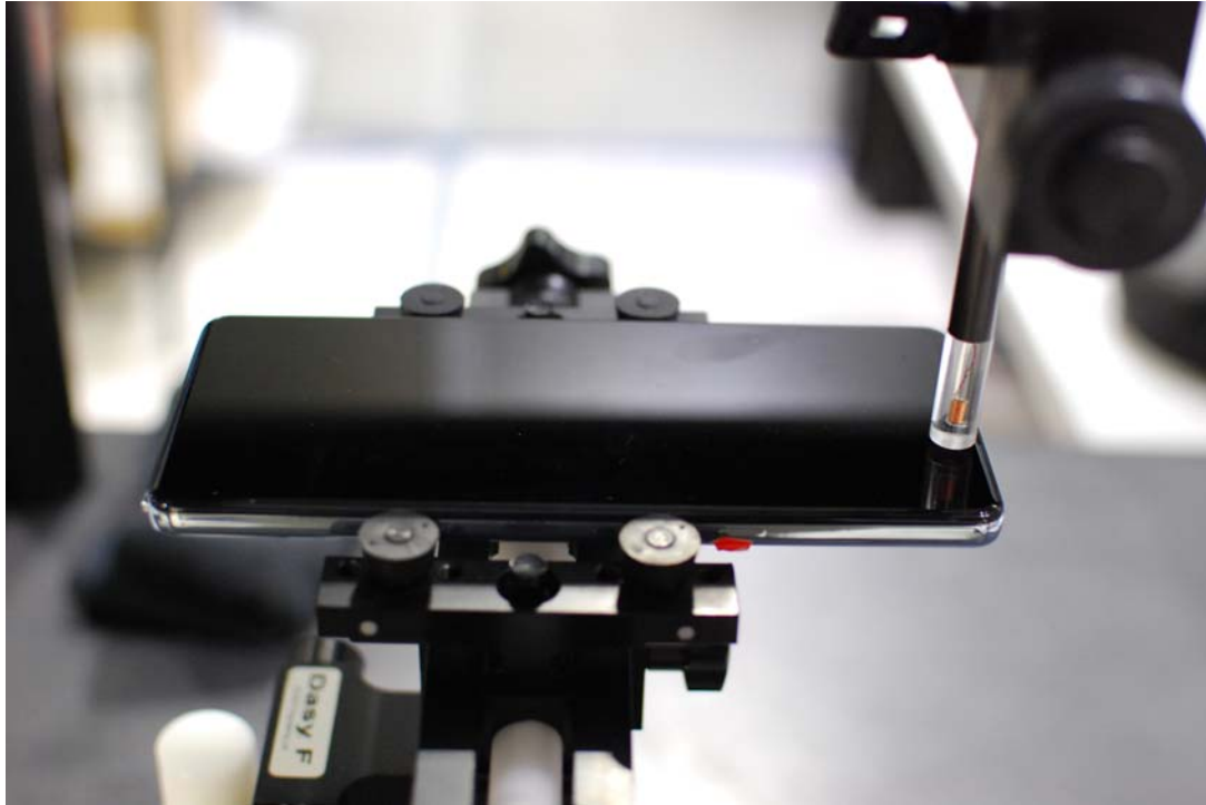
Figure 16-1 Test Setup for Wireless Device
