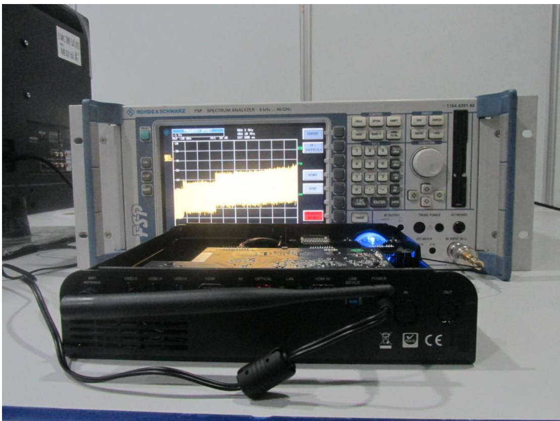
Conducted Test setup photo
