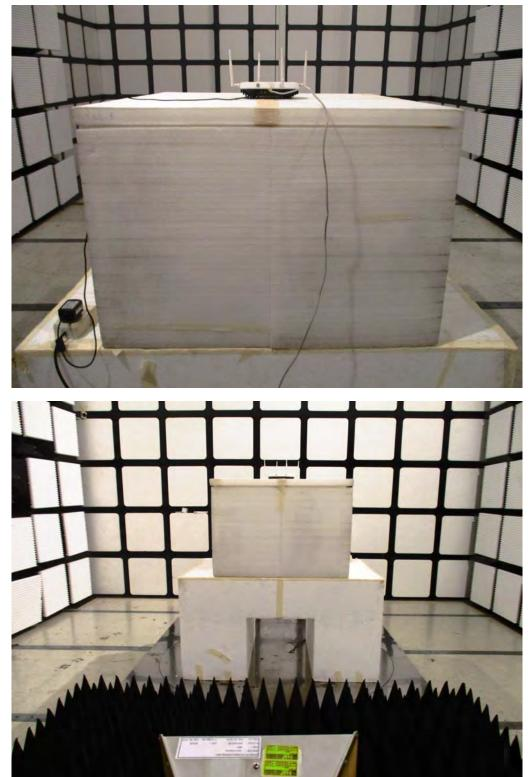
Test Mode 7: EUT 1 + Set 9 Dipole Antenna / 4.67 dBi
