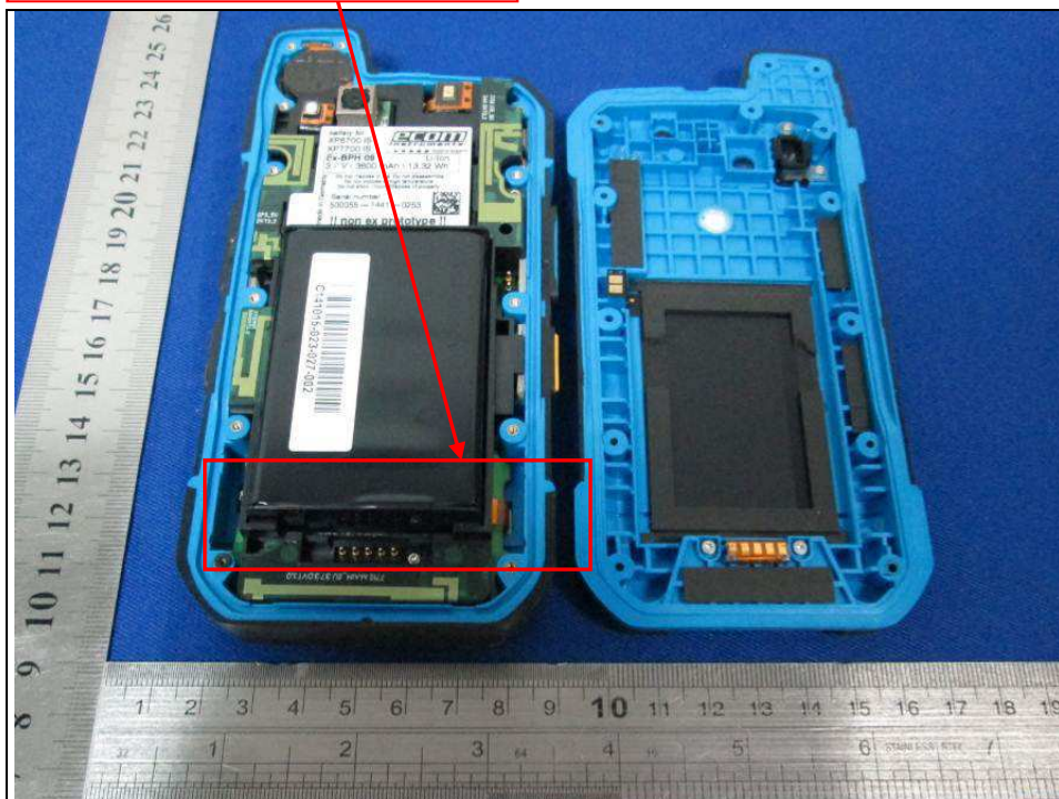
WWAN Main TX/RX Antenna
