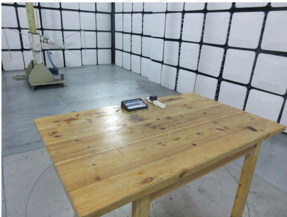
Photo of Radiation Emission Test
