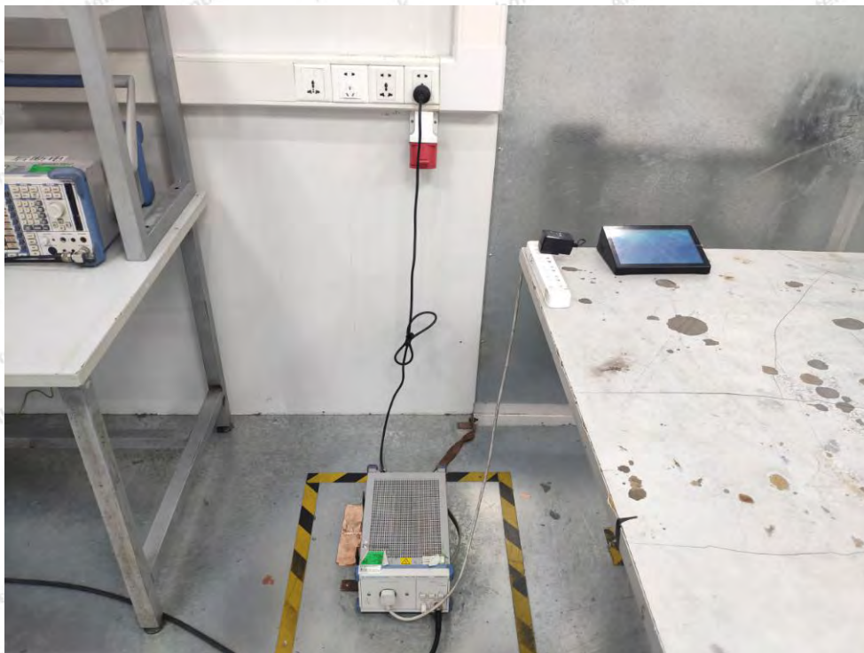
Photo of Conducted Emission Measurement
