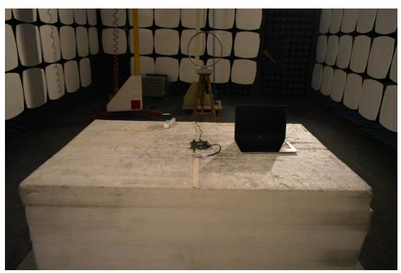
3. Radiated emission (9KHz-30MHz)
