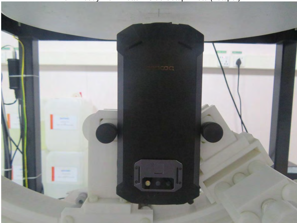
10mm body-worn Bottom Side Setup Photo (hotspot)
