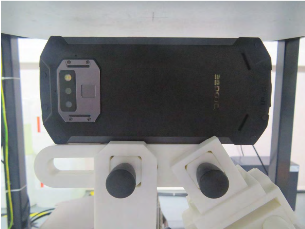
10mm body-worn Left Side Setup Photo (hotspot)
