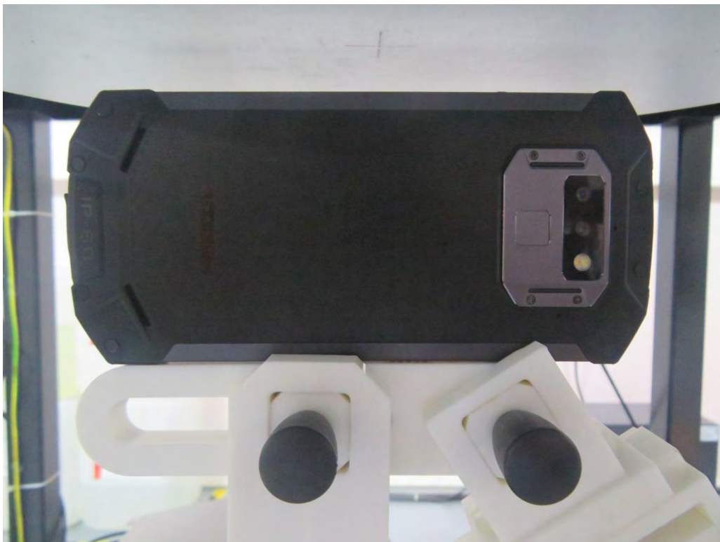
10mm body-worn Right Side Setup Photo (hotspot)
