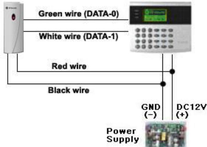
Figure: External Reader Connection
