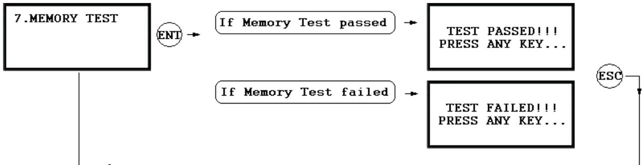
. If the Data Memory has problems, LCD will show the Memory failure message. In this case, contact manufacturer for technical support.
