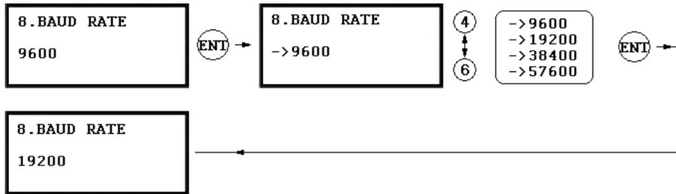
. GE313 supports 9600, 19200, 38400 and 57600bps of Baud Rate and default Baud Rate is 9600bps. Wrong Baud Rate setting will cause communication error and you have to set same Baud Rate for the same communication network.
