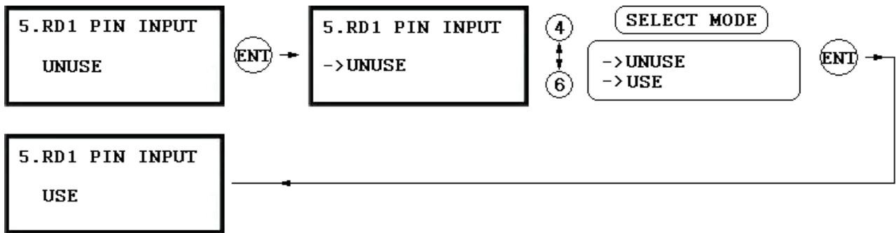
. This function is for USE/UNUSE the keypad inputs for the Reader#1. The default setting is UNUSE the keypad inputs. If you want to access the door by entering the user ID by keypad, set this mode USE. You have to set this mode USE when the unit is operating with Password.
