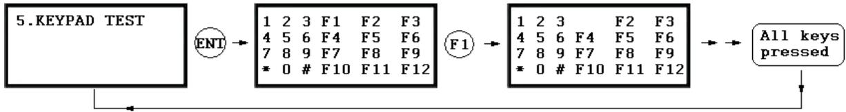
. LCD will display all keys of the unit. Press each key from the keypad one by one, the depressed key will disappear from the LCD. Note that ENT key is “#” and ESC key is “\*” on the LCD.
