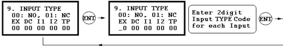
. You can program input type(00: NO, 01: NC) to each Input. The default input type is “00” which means input is NO type.
