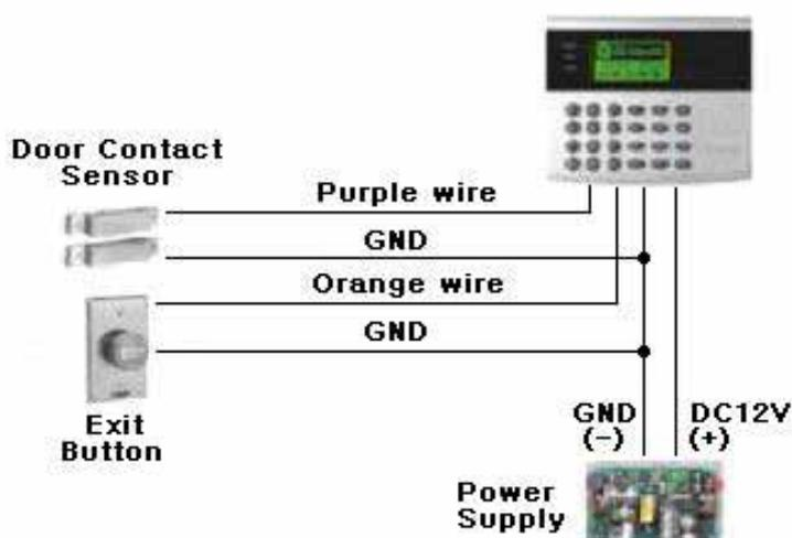
Figure: Input Device Connection
