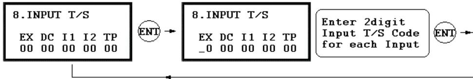
. You can link a T/S Code to each Input. The default T/S Code is “00” which means no T/S is applied to the Inputs. This setting is very useful when you want to activate PIR sensor input for a Time Interval.
