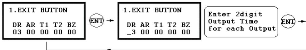
. You can program OUTPUT activating time when the EXIT button pressed. The value put here is value x second when the Time Unit set to 1 second and value/10 second when the Time Unit set to 0.1 sec. You can set the time from 00 to 98 seconds (0.0 to 9.8 seconds if Time Unit set to 0.1 sec.) and if you put the value “99”, the Output will activate forever until you reset the Output.
