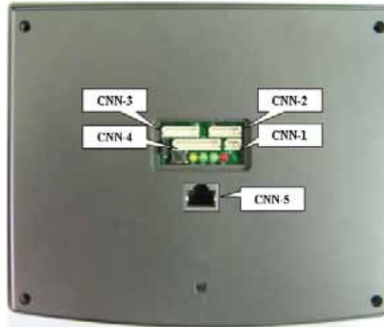
Figure: Connector Layout
