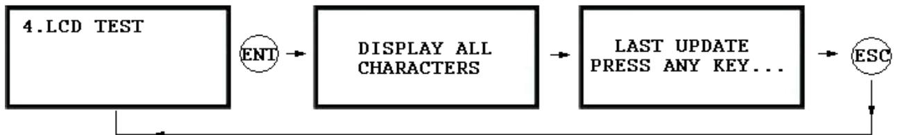
. The LCD will display all characters on the screen. When the test is done, the LCD will show “Last Update Press any key”.
