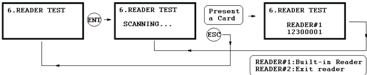
. LCD will display “Scanning...” for reading the cards. Present the card to one of the readers.
