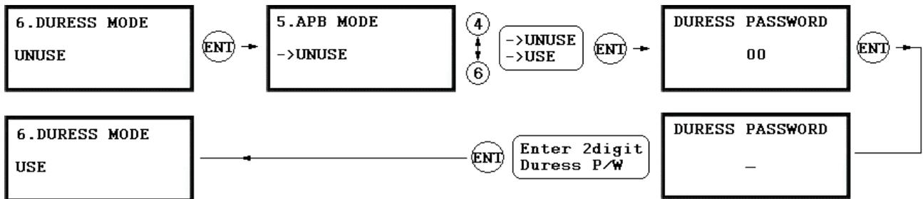
. You can set Duress Mode for Reader#1. Default setting is UNUSE. If you select USE, LCD will display default Duress Password '00'. Enter 2 digit Duress Password.
