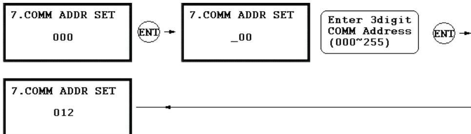
. The default Communication Address is “000” and set a different COMM Address for each unit in the loop.
