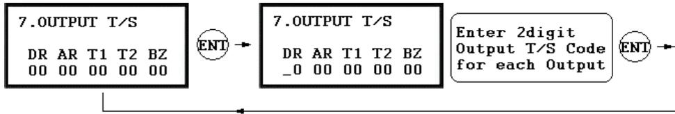
. You can link a T/S Code to each Output. The default T/S Code is “00” which means no T/S is applied to the Outputs. This setting is very useful when you want to open the door for a Time Interval.
