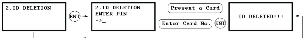
. Registered ID will be deleted in the controller by presenting the card or input the ID number from the keypad. Present the card to be deleted. The ID number will appear on the LCD. If you don't have the card, input 8digit ID number and <ENT> key from the keypad. If the ID number is found, the ID will be deleted and display "ID DELETED". If the ID number is not found, the display will show "UNREGISTERED ID". You may repeat ID DELETION many times.
