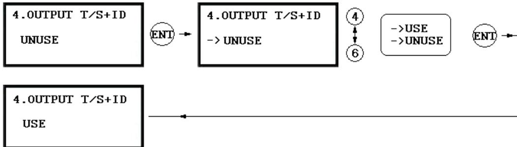
. Output Time Schedule+ID is to unlock the door when the first user grants the access during the Time Interval of the Time Schedule. The door will be locked just after the Time Interval period is over.
