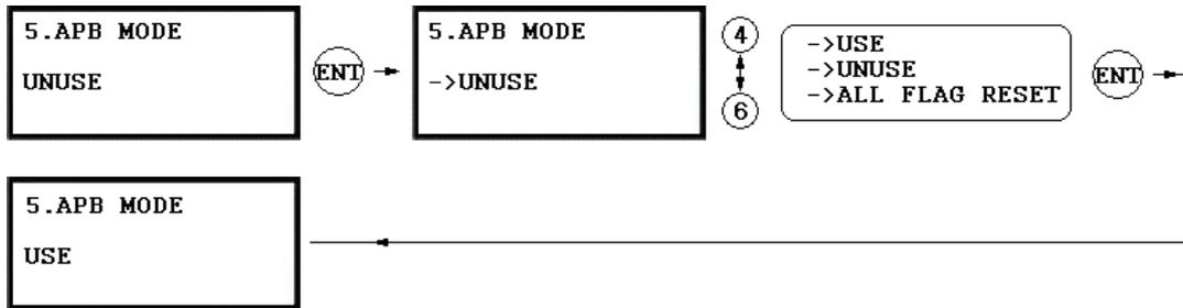
. The Anti-pass Back mode is only used when you installed Exit Reader. Do not set this mode in USE when you installed Exit Button. You must install GE313 for entry and Exit Reader for Exit.
