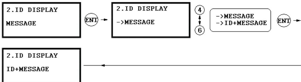
. This function is to set display mode. If you want to display user ID number on the LCD, select ID+MESSAGE. MESSAGE: Text message and "\*\*\*\*\*" characters will be displayed on the LCD and it will not display user ID number. ID+MESSAGE: The user ID number will be displayed on the LCD with text message. Default setting is MESSAGE only.
