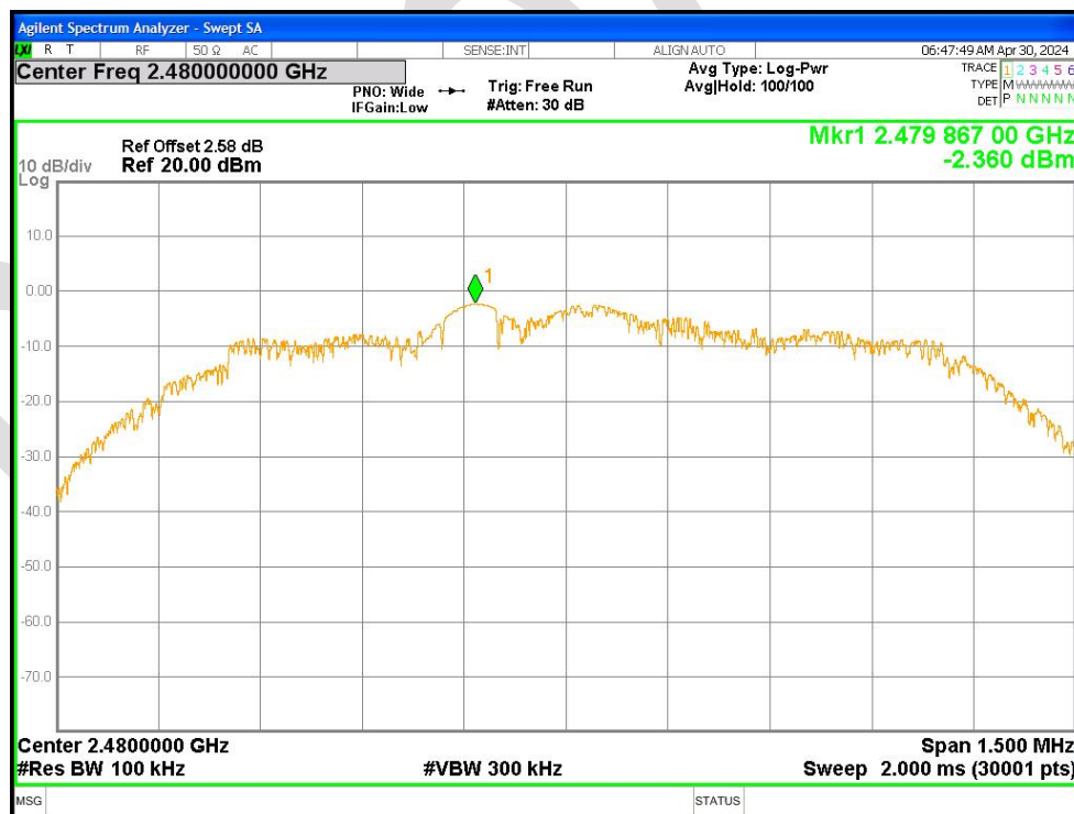
Tx. Spurious NVNT 2-DH1 2480MHz Ant1 Emission
