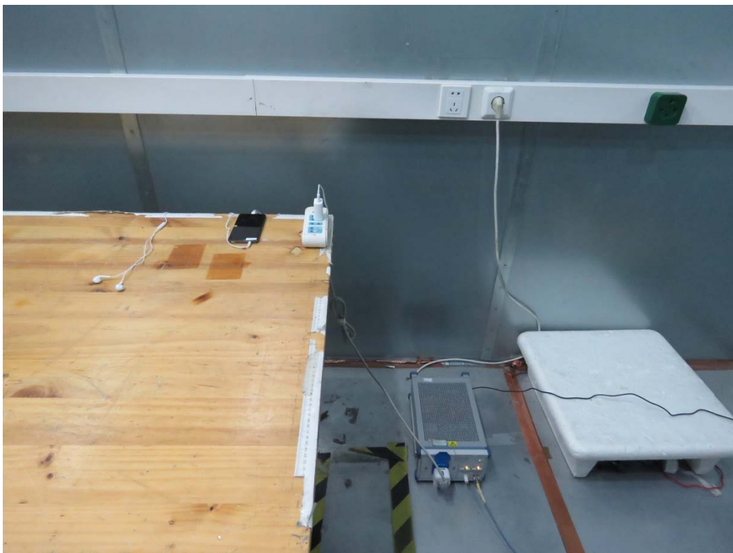
Picture 2 Conducted Emission Test Setup
