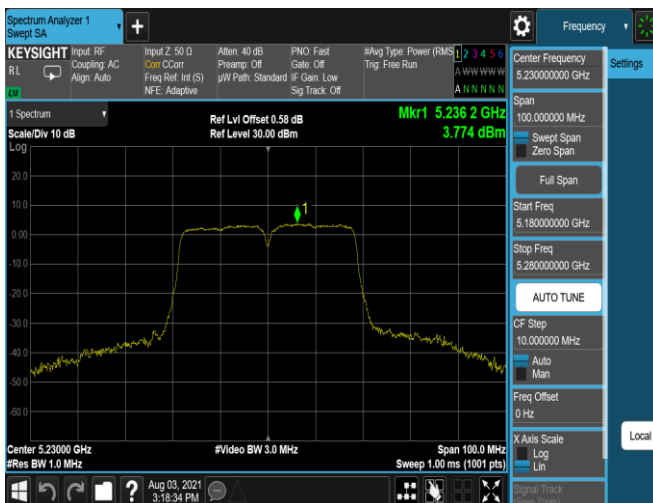
Plot 7-303. ISED PSD Antenna 5T (40MHz BW 11n - Ch.46, MCS5)
