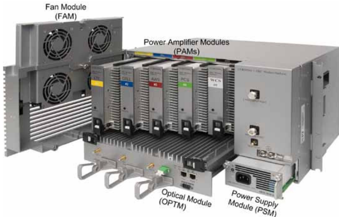
Figure 2-13 MRU Main Modules
