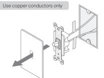
Ground: Usually green or copper. Neutral: Usually white and not connected to the dumb switch. Line: Usually black and coming from the circuit breaker. Load: Usually black. One end is connected to the light. If you are unsure, consult a qualified electrician.
