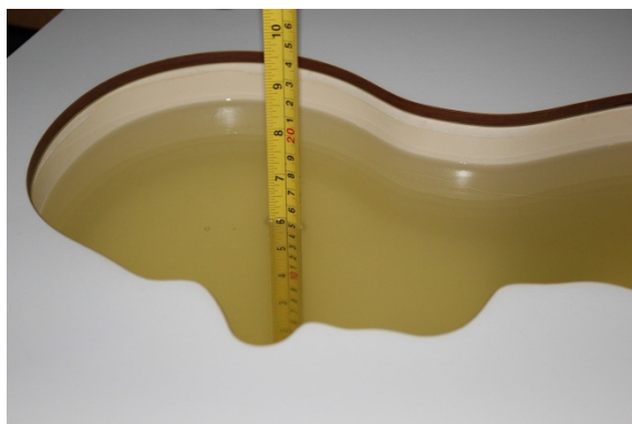
Liquid depth in the head phantom (1750MHz)
