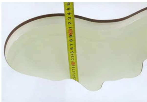
Liquid depth in the head phantom (1900MHz)
