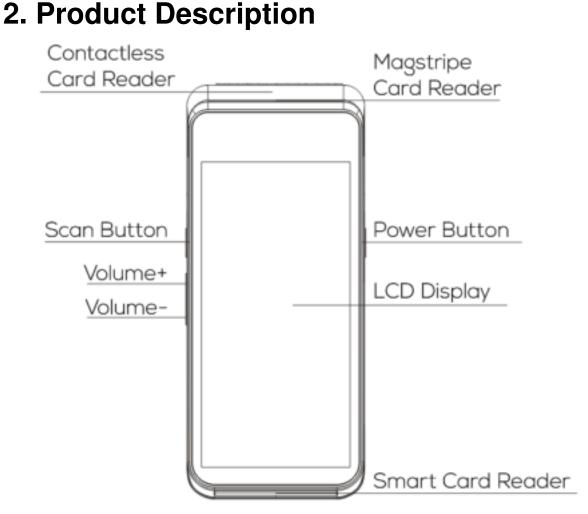
Contactless Card Reader, Scan Button, Volume+, Volume-, Magstripe Card Reader, Power Button, LCD Display, Smart Card Reader
