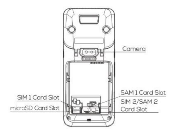
Scanner, SAM 1 Card Slot, SIM 2/SAM 2 Card Slot, SIM 1 Card Slot, microSD Card Slot
