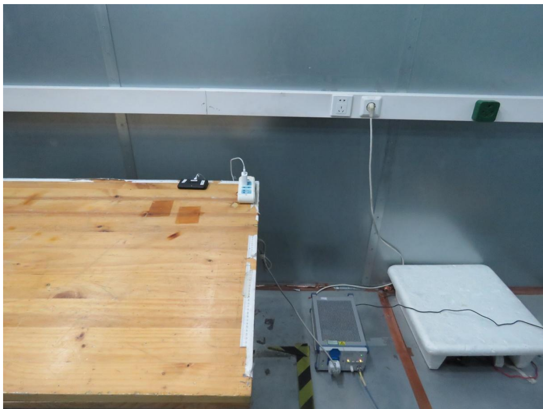
Picture 2 Conducted Emission Test Setup
