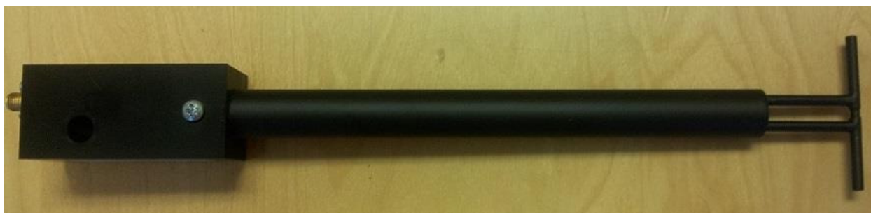
Figure 1 – MVG COMOSAR Validation Dipole
