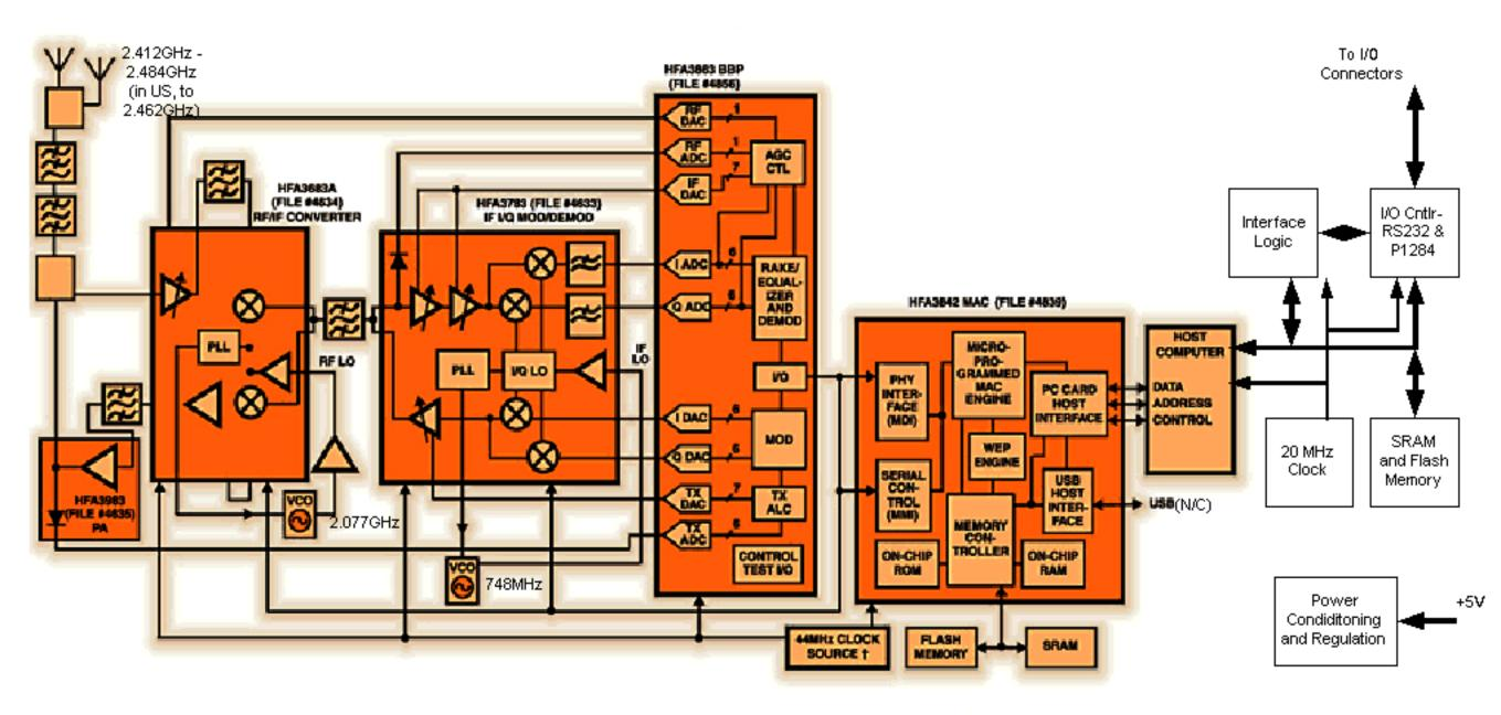
† THE HFAS842 MUST BE SUPPLIED WITH A SEPARATE 48MHz CLOCK WHEN USB IS USED.
