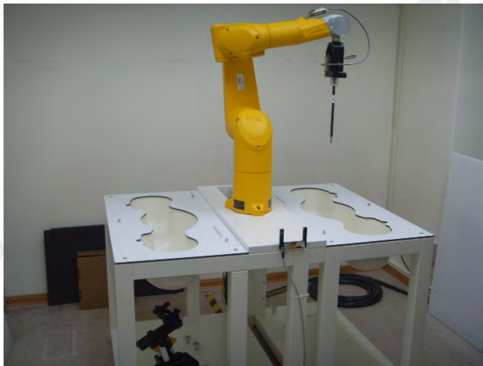
Fig.1 Photograph of the SAR measurement system
