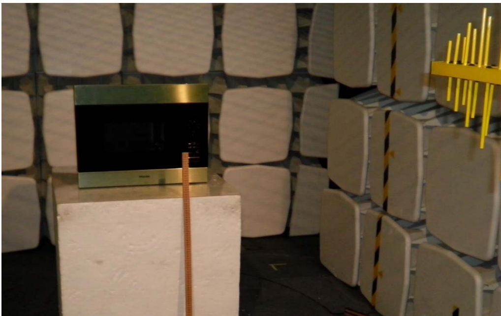
Photograph 5.7.2 Radiated emissions testing 30MHz-1GHz (Anechoic chamber)
