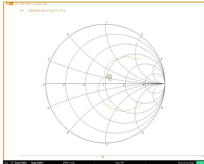
FIGURE 7 SMITH CHART - TUNED BT ANTENNA (LENGTH REDUCED BY 0.1MM)
