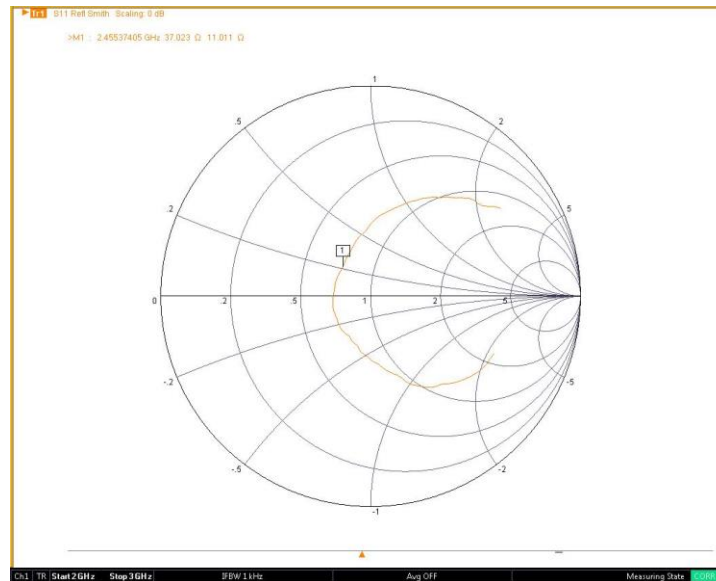
FIGURE 5 SMITH CHART -UNMODIFIED WI-FI ANTENNA
