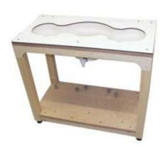
evaluation of left and right hand phone usage as well as body mounted usage at the flat phantom region. Reference markings on the phantom allow the complete setup of all predefined phantom positions and measurement grids by manually teaching three points in the robot.
