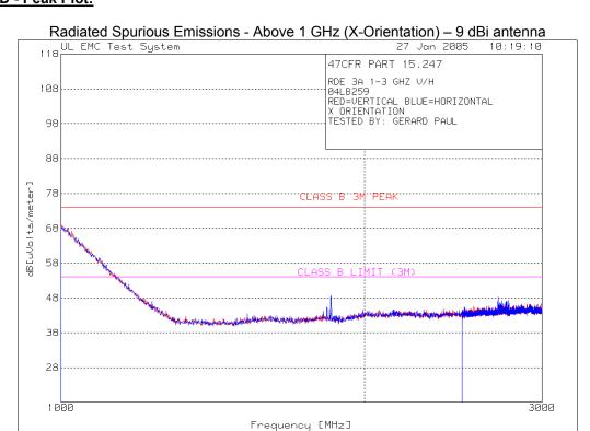
Note: Broad emission from 1000 to 1400 MHz is due to mathematical correction for high-pass filter loss. No spurious emission was observed in this band.
