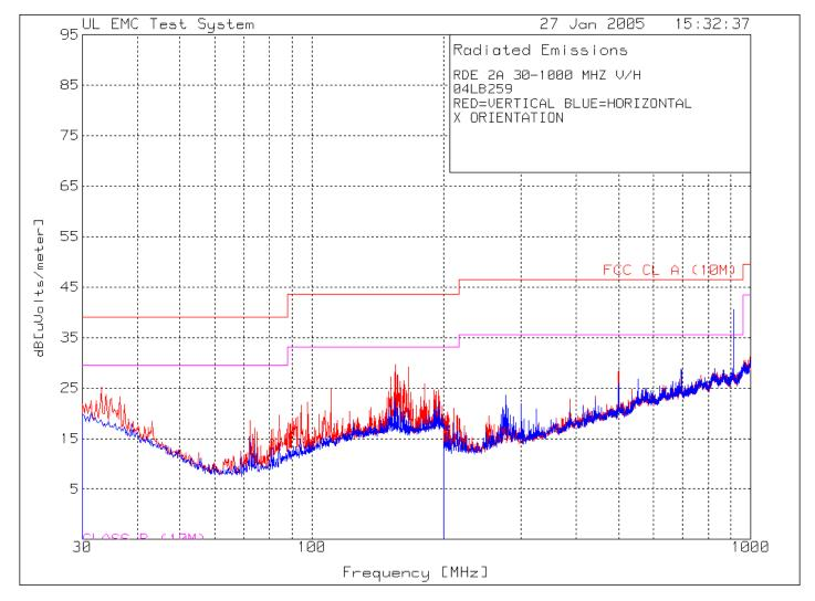
Note: Measurement performed at 10 meter distance with Class B limit extrapolated as 20 dB/decade. Emission from transmitter local oscillator in 902-928 MHz band is disregarded.
