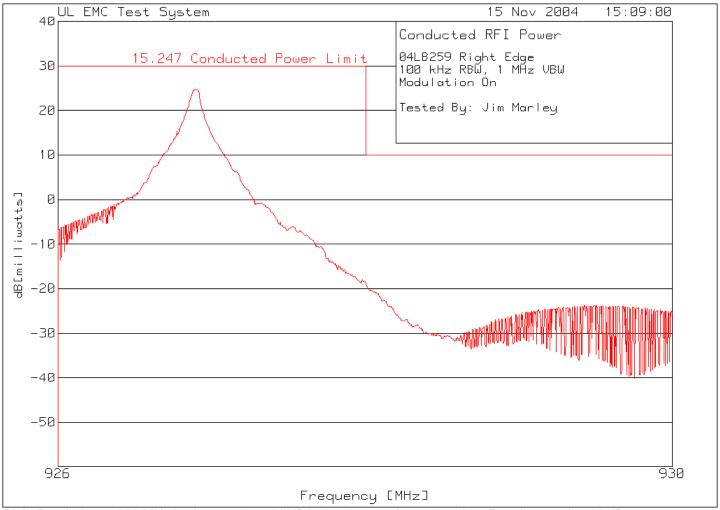
Right Bandedge at 928 MHz is shown to be >30 dB below lowest channel carrier. Requirement is >20 dB.
