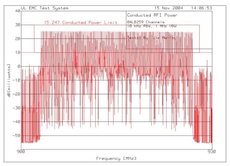
The device is shown to have 120 hopping channels.
