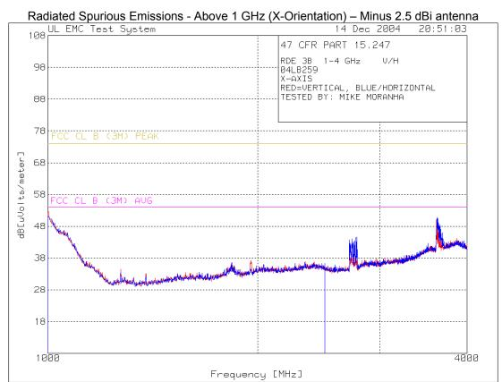
Note: Broad emission from 1000 to 1400 MHz is due to mathematical correction for notch filter loss. No spurious emission was observed in this band.
