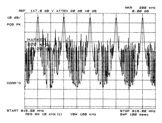
Channel spacing is 200 kHz center to center.
