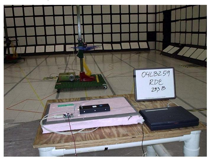
Note: Styrofoam added below EUT to reduce reflection of emissions from wooden tabletop at high frequencies. EUT is shown in the "X Orientation" or flat. Antenna is positioned to be pointed with direction of maximum gain toward receive antenna. Measurements were also performed with EUT positioned on side and on end as shown below:
