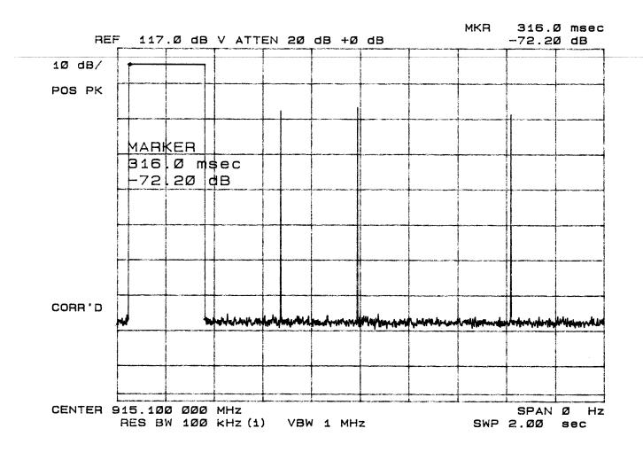
Hop duration is 316 milliseconds at any channel.
