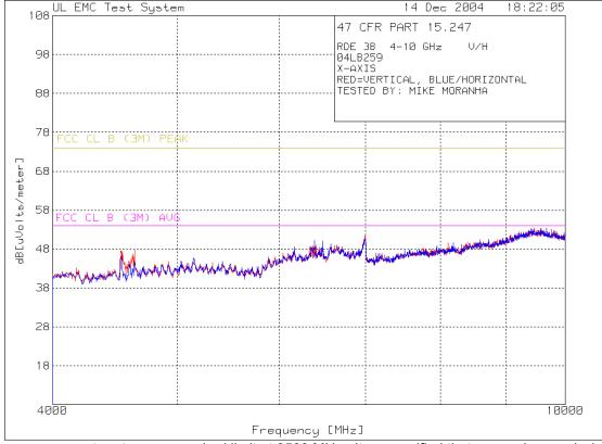
Note floor for measurement system approached limit at 9500 MHz. It was verified that no spurious emission was present by repositioning receive antenna to a 1 meter distance with no increase in emissions observed.
