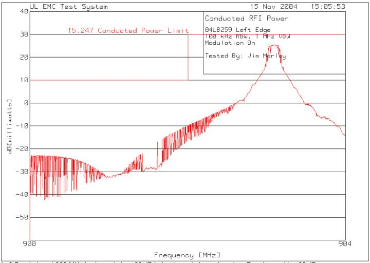
Left Bandedge at 902 MHz is shown to be >30 dB below lowest channel carrier. Requirement is >20 dB.
