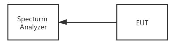
The EUT is connected to the Spectrum Analyzer; the RF load attached to the EUT antenna termina is 500hm; the path loss as the factor is calibrated to correct the reading. Tune the measurement with the spectrum analyzer's resolution bandwidth (RBW) = 100 kHz. In order to make an accurate measurement, the span is set to be greater than RBW.
