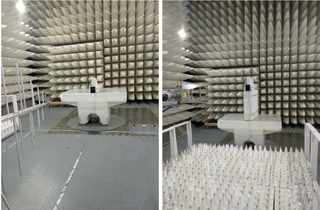
Photograph 8.2.1 Setup for radiated emission measurements, general view
