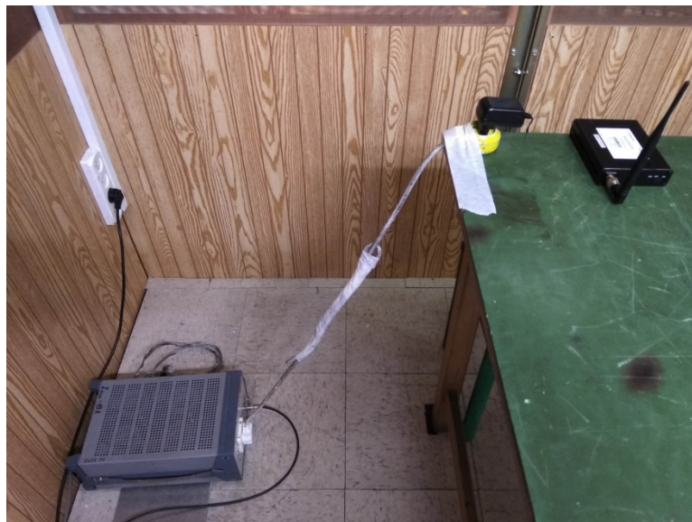
Photograph 8.1.1 Setup for conducted emission measurements
