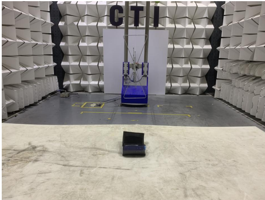
Radiated spurious emission Test Setup-1(Below 1GHz)
