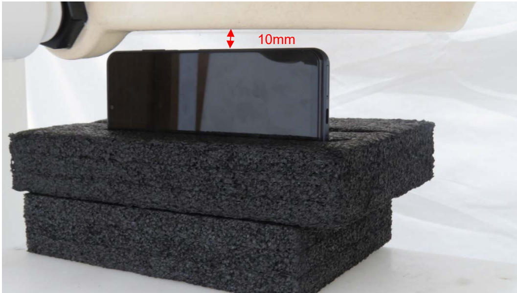
Picture 13: Right Edge, the distance from handset to the bottom of the Phantom is 10mm
