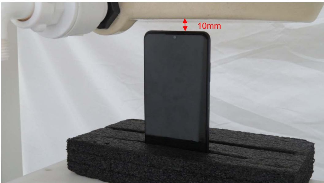
Picture 14: Top Edge, the distance from handset to the bottom of the Phantom is 10mm
