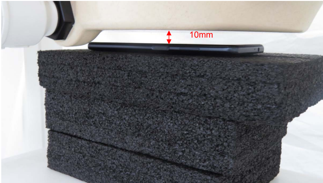
Picture 11: Front Side, the distance from handset to the bottom of the Phantom is 10mm
