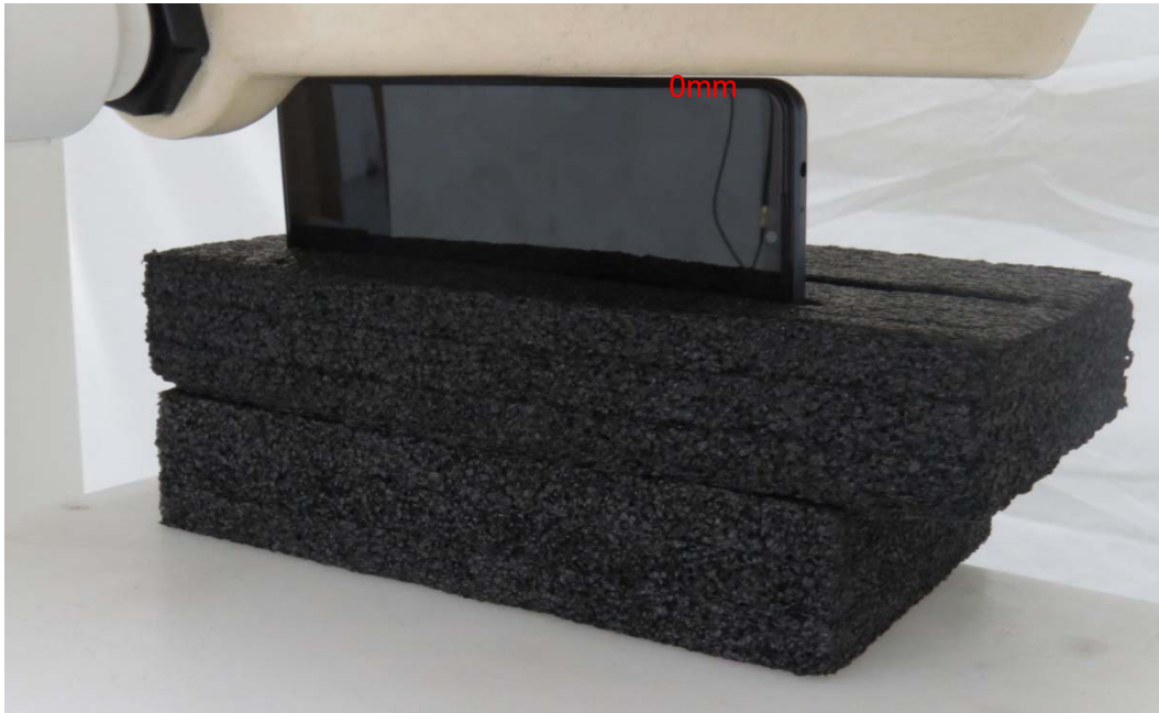
Picture 17: Left Edge, the distance from handset to the bottom of the Phantom is 0mm
