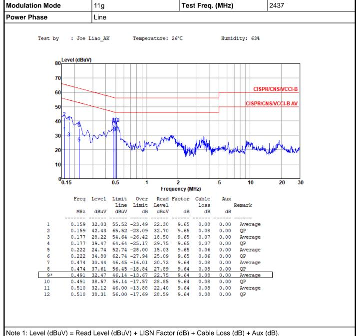
Note 1. Level (ubuv) = Read Level (ubuv) + Lishi Factor (ub) + Cable Loss (ub) + Aux (ub)
