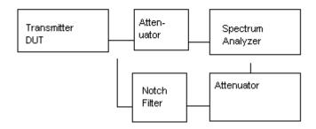
Method of Measuring Conducted Spurious Emissions
