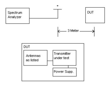
Equipment placed 80cm above ground on a rotatable platform.
