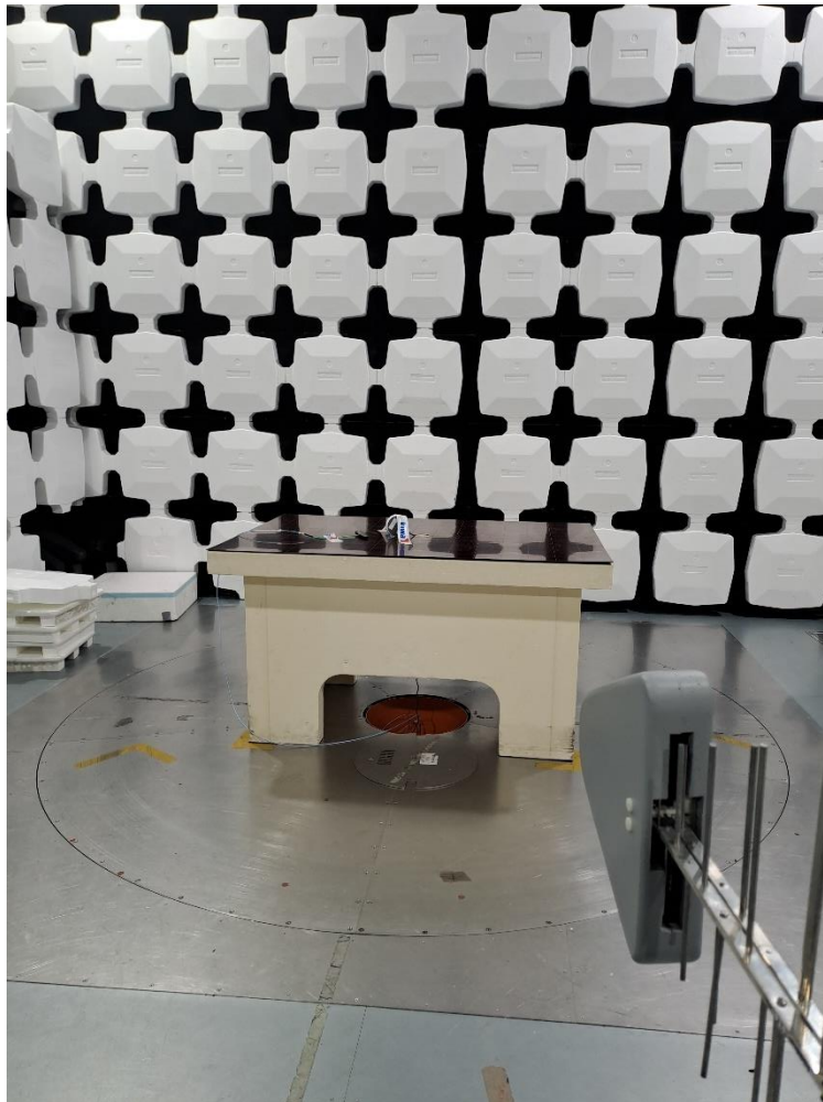
Photo 2 Photograph test setup radiated emissions 250-1000 MHz, report section 3.1
