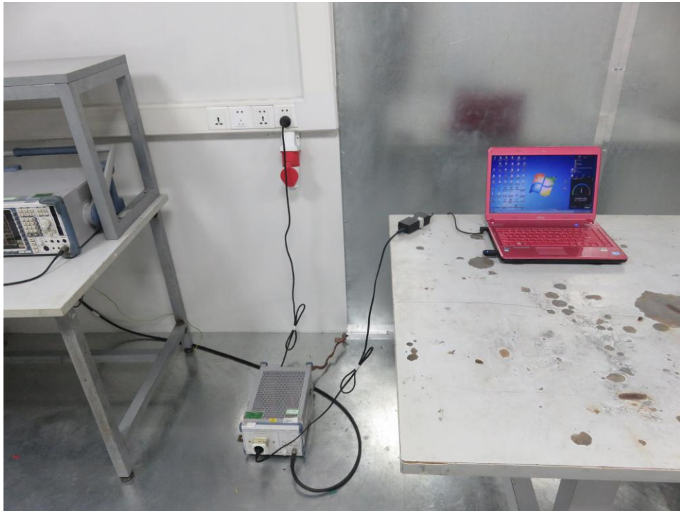
Photo of Conducted Emission Test
